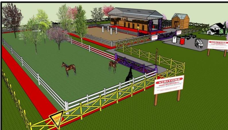
This figure demonstrates the different biosecure zones. The yellow perimeter fencing creates a controlled access zone. Restricted access zones, like paddocks and stables, are marked in red. Controlled access points are shown in purple.
